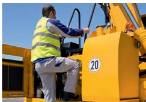
A new, straight service access ladder, newly designed, large tool boxes and a separate compartment for the refueling pump.
