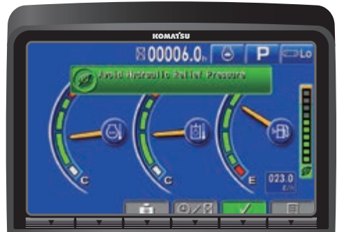
Features like ECO-gauge, a fuel consumption gauge and idle caution all assist to further reduce fuel consumption.
